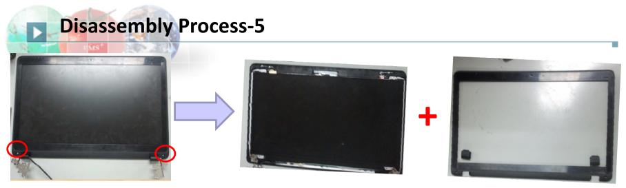
Loose screw and screw mylar, take off hinge cover and lcd bezel.
